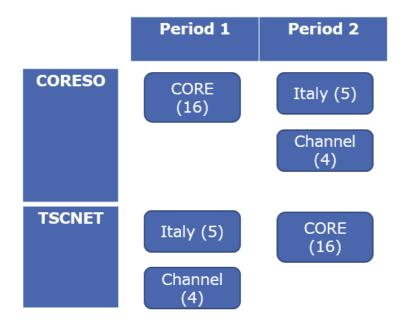
The advantage of the setup is that only 3 desks will be required across 2 RSCs, while the disadvantages are: no immediate backup, high workload for one RSC and RSCs need to build expertise on the whole CCR.
