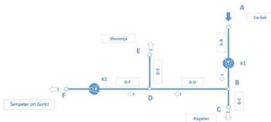
Figure 1: Scheme of the Slovene transmission system.
