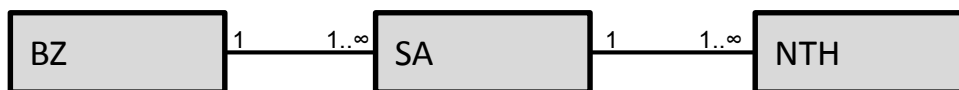
Figure 7 Relations between bidding zone and scheduling area, and scheduling area and NEMO trading hub
